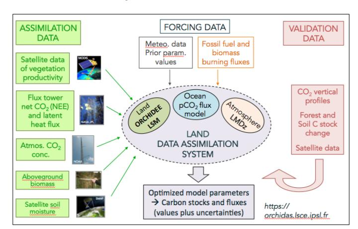
CCDAS scheme coupling ORCHIDEE & the LMDz atmospheric model: Assimilation of multiple data streams related to C/W/E budgets; To correct model parameters and initial state
